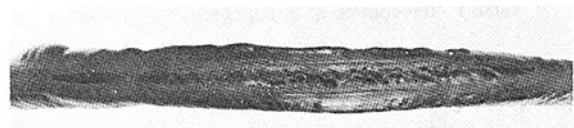
Fig. 6 CN2 seal after test (rating 1)
